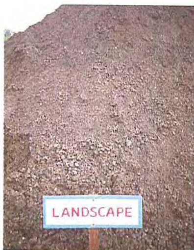
SMARTscape Mix: A top quality landscape mix incorporating 70% high quality loam, 20% 'Dillo Dirt and 10% coarse grit sand.
