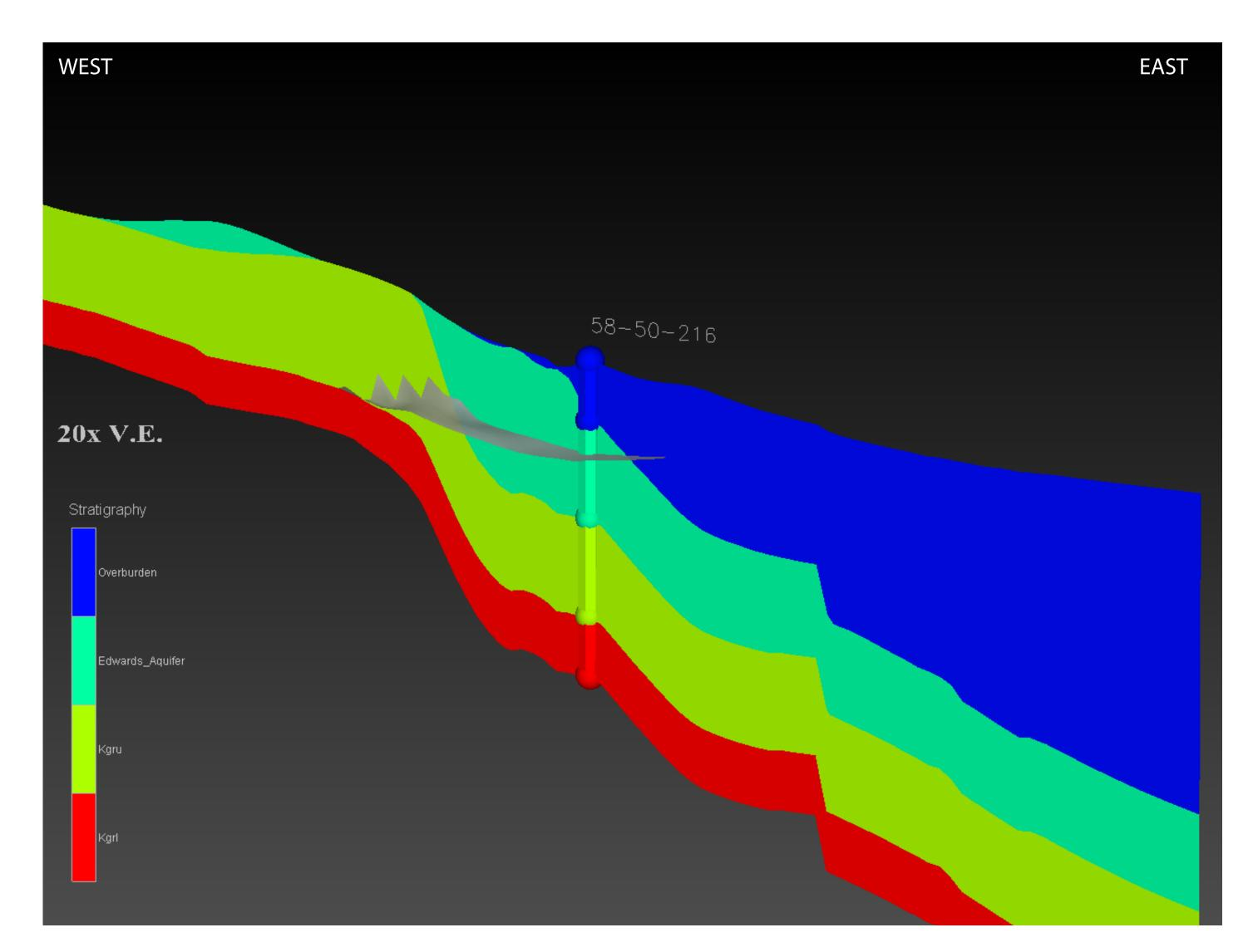
Oblique view of the geologic cross section (west to east) through the Target Well. Cross section from regional model. March 2009 potentiometric surface is denoted as gray shading.
