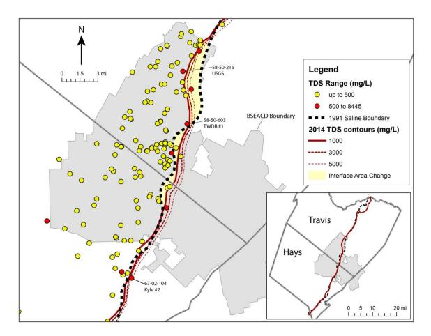
**Figure 5.** Map of wells that show a range of measured and estimated TDS values. Wells noted in the text are labeled on the map. The well on the southwest portion of the study area is likely influenced by completion of the well in a portion of the Trinity Aquifer, often a source for elevated TDS.
