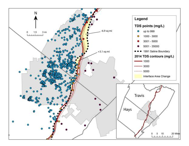
**Figure 4.** Results of assimilated composite TDS data from wells completed in the Edwards Aquifer and the resulting delineation of the freshwater/saline-water interface. There is a mapped apparent net loss of 3.8 mi<sup>2</sup> of freshwater aquifer when compared to the 1991 saline boundary delineation.
