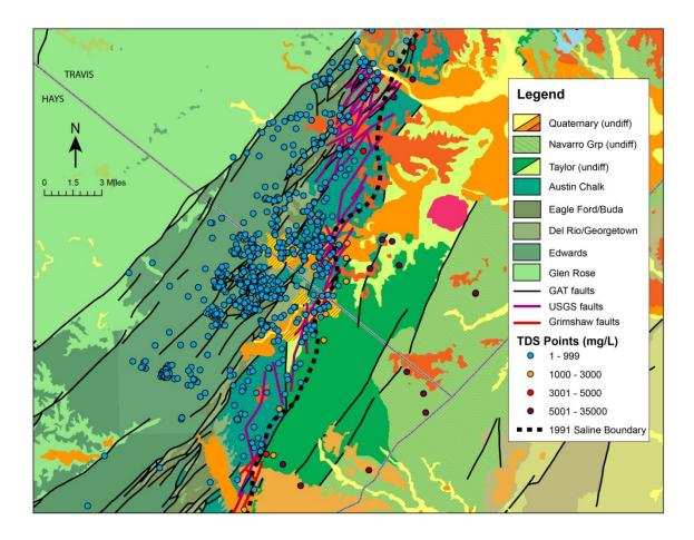
**Figure 2.** Geologic map of a portion of the study area showing previous saline boundary and also faults mapped in the study area. TDS values from this study are plotted that show a need to revisit the boundary delineation. The geology is modified from the Geologic Atlas of Texas (GAT).
