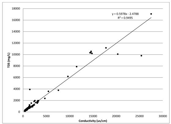
Figure 3. Correlation between measured total dissolved solids and specific conductivity.
