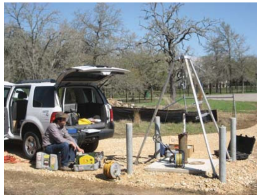
16-3 Photograph showing the winch and tripod used to raise and lower the wireline tool that measures pressures in each zone. The same tool also can collect up to 1 liter of sample from each zone. Photo by Brian B. Hunt.
