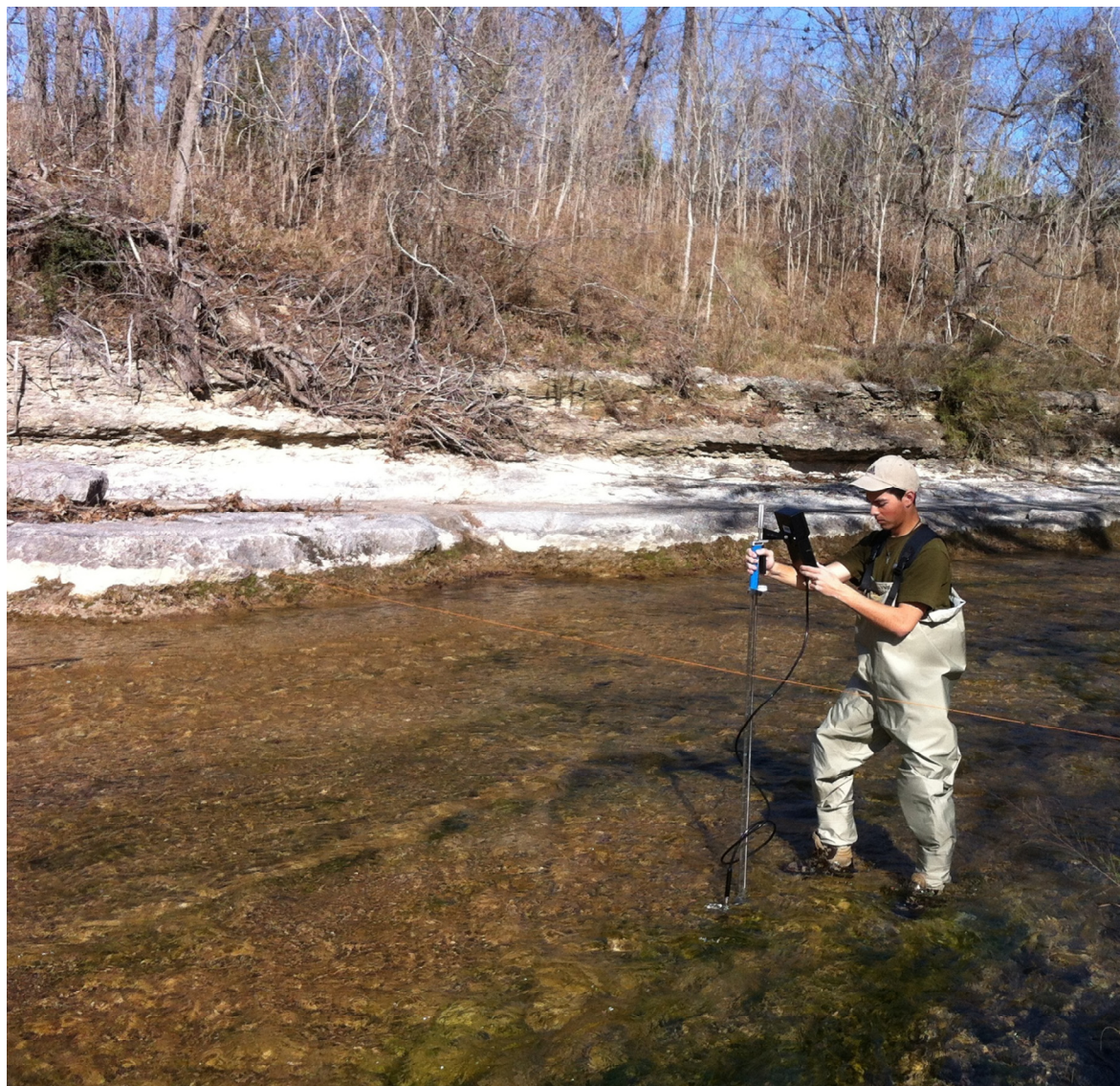
Figure 4. Photo of wading flow measurement using the FlowTracker instrument at the Onion Creek at FM 150 (USGS site). Photo taken 1/6/15.
