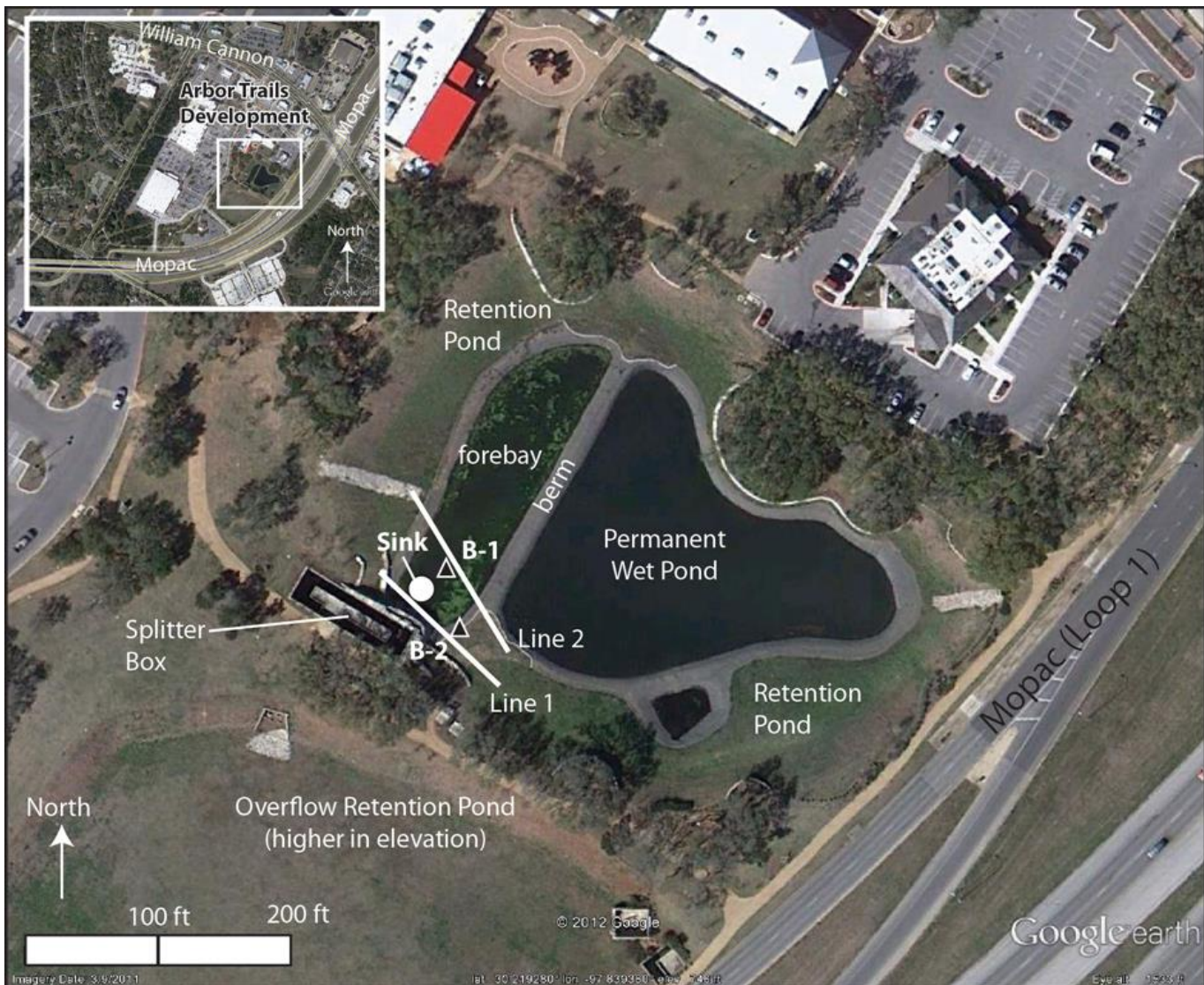
Figure 3. Detailed site map with key elements of the stormwater retention pond (SWRP), sinkhole location, and 2012 geophysical lines and boreholes.
