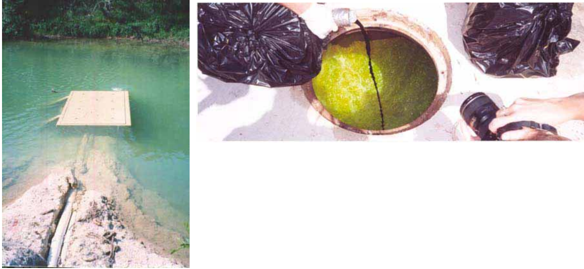
Figure 2. Concrete vault and valve system above Antioch Cave within Onion Creek (left). Sodium fluorescein dye being poured into the top of the vault (right).
