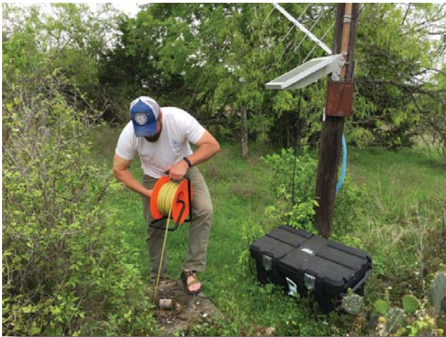
Figure 4: BSEACD staff uses an eline to take a water level measurement to calibrate the pressure transducer at the Hoskins well. This site has telemetry, so water level data are transmitted to the web.
