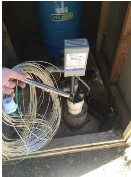
Figure 1: Monitor well equipped with a pressure transducer.
