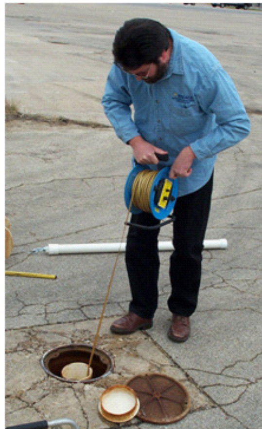
Figure 5: Picture of staff measuring the depth to water in a well with an eline.
