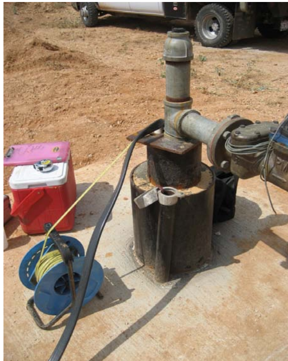
Photograph of water-level monitoring with an e-line during KBDJ Quarry Middle Trinity pumping test.
