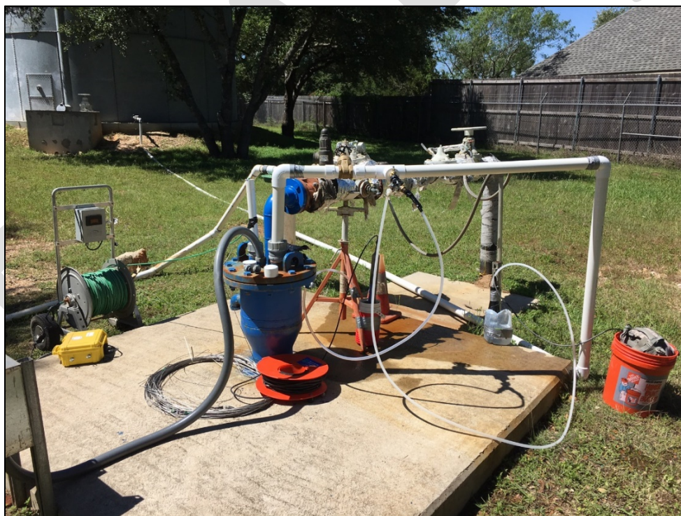
Figure 4. Photograph of RRWSC#5 ASR test well. Temporary PVC pipe was used to inject stored Edwards Water. Also shown are the equipment used to measure water levels and field parameters. The storage tank in the distance holds Edwards water prior to injection.
