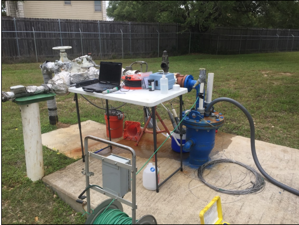
Figure 5. Photograph of RRWSC#5 ASR test well equipped for continuous water level and field parameter measurements.
